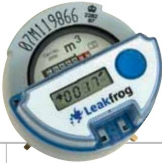
The function of the Leakfrog is to detect, store and display the maximum time between successive pulses from pulsed output meters. The maximum time between pulses is the reciprocal of minimum observable flow. **The higher the value displayed on the Leakfrog, the smaller the leak.**
